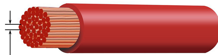
Max strand diameter: 0,4mm Max strand area: 0,125mm 2 / 26 AWG
