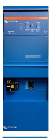
The VEP (Victron Electrical Panel) makes for an easy and simpler installation connecting in one location all the AC and DC cabling for a Victron inverter/charger. The Primary VEP has a Bypass Assembly to isolate the battery-based system allowing for safe inspection and maintenance of system while still powering the load panel with an AC source. This is a code compliant solution (UL and CSA) comporting to UL 1741 and CSA C22.2 for standards for safety.
