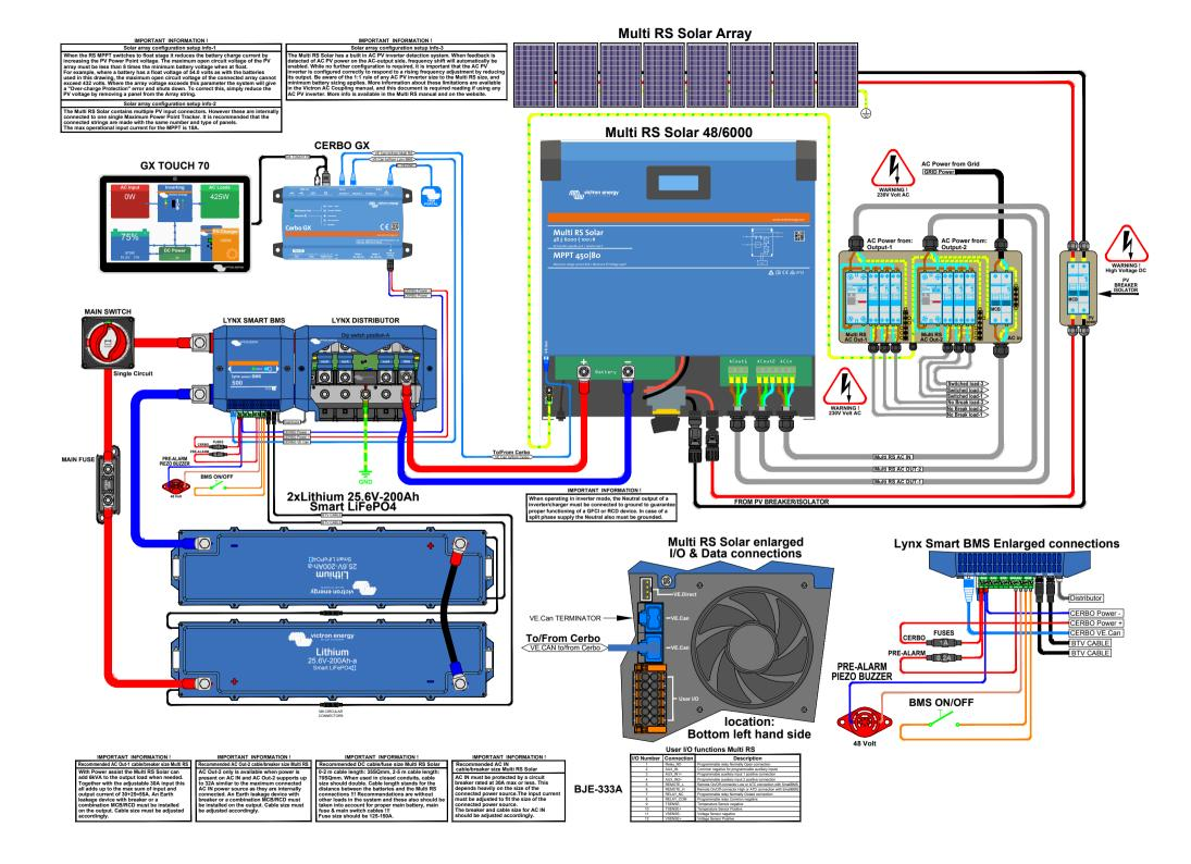
from the Main switch Positive power continues to the Positive battery power connection of the Lynx Smart BMS. Negative power from the top visible Li battery runs to the Negative battery power connection of the Lynx Smart BMS.
