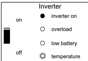
The internal temperature is reaching a critical level.
