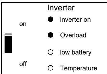
The inverter is switched off due to overload or short circuit.
