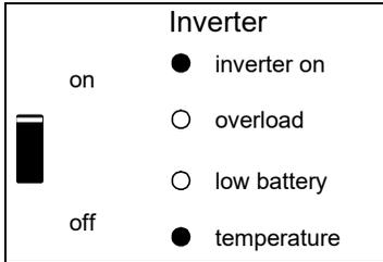
The inverter has switched off due to the electronics temperature being too high.
