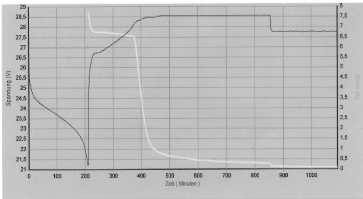
The graph shows the discharge-charge curve of a 24V 210Ah battery
